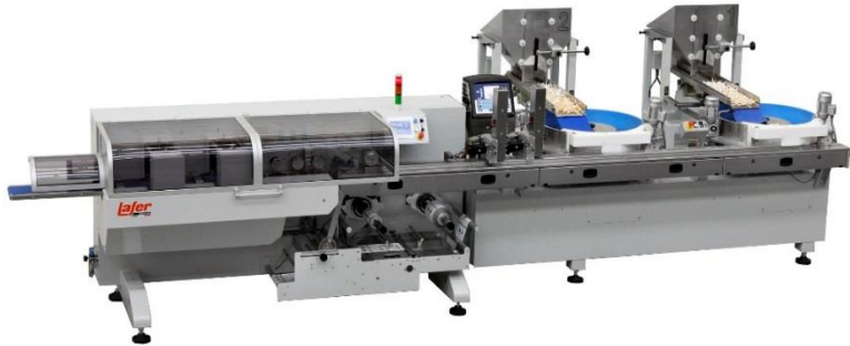
Special h.f.f.s. machine for twin-wrapping of lolly pops strips
