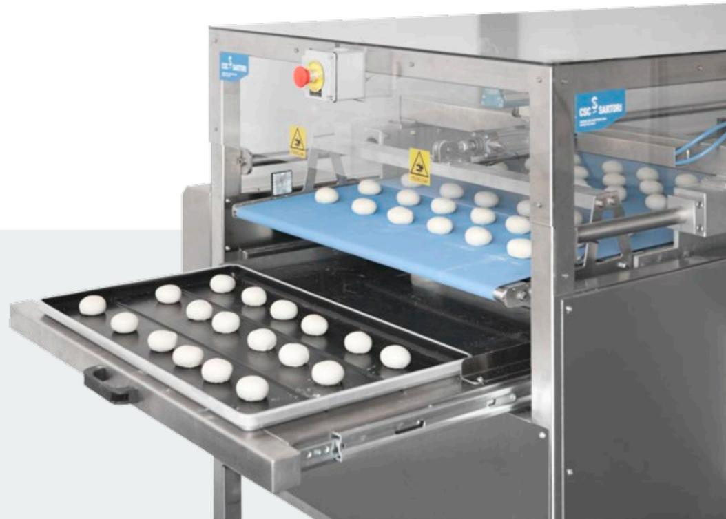
The retractable conveyor belt for tray loader is a device which receives the dough pieces from the in line machine, place them into the waiting tray which will be removed manually.
